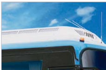
Roof on cooler (BH090)
