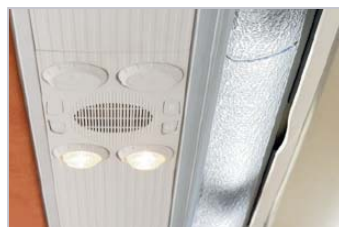
Air conditioner louver / lamp
